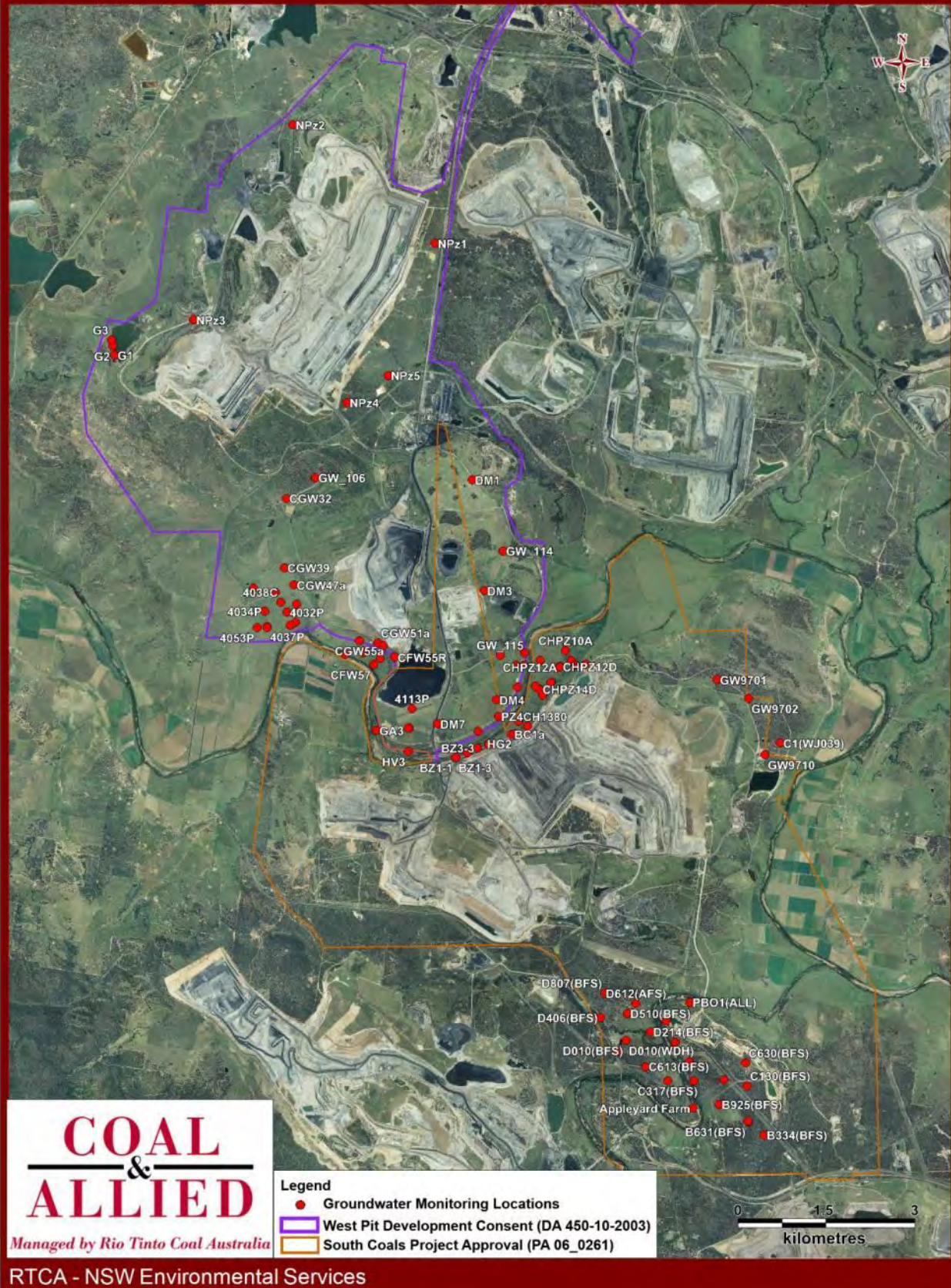
Figure 77: Groundwater Monitoring Location Plan
