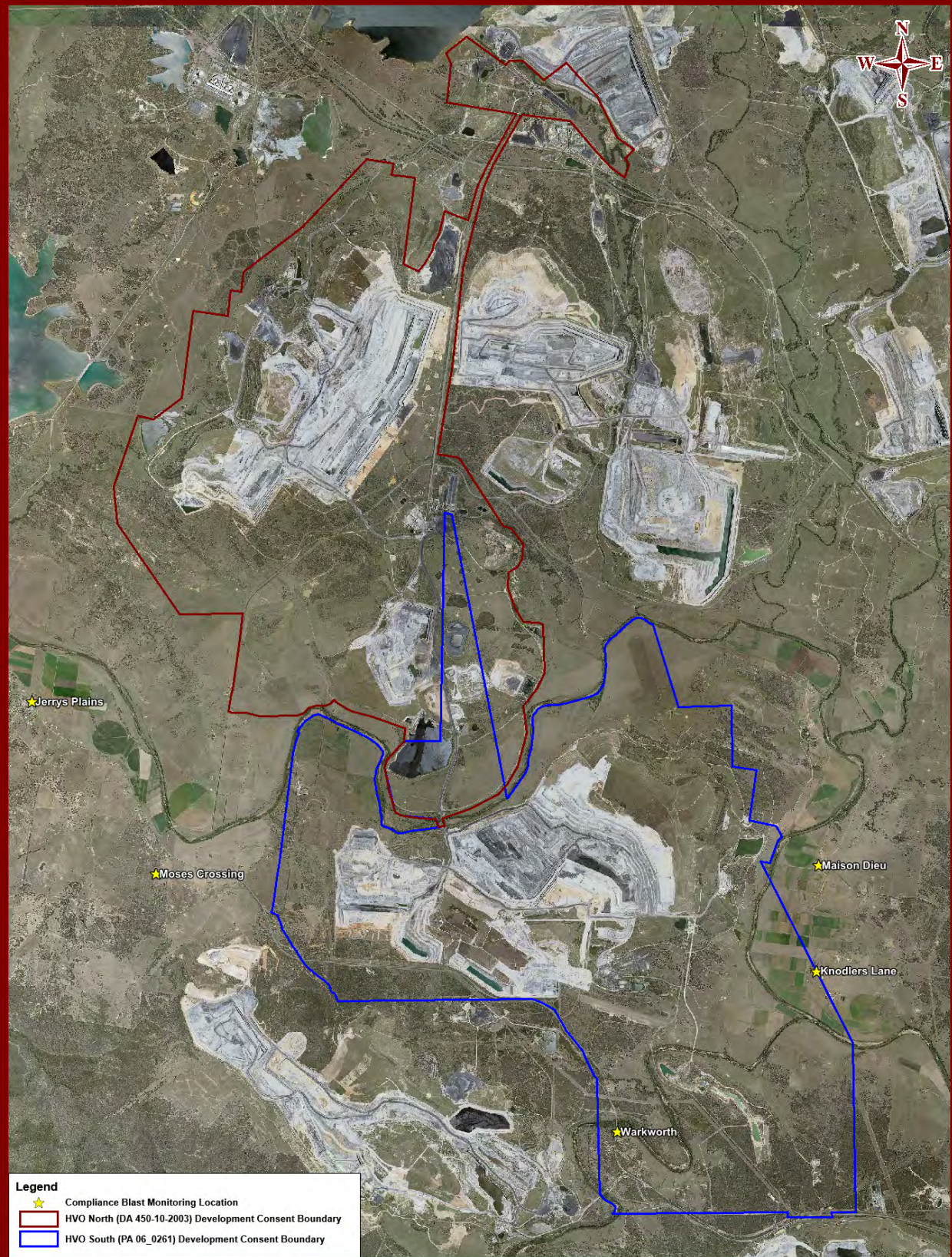
Figure 15: Blast Monitoring Location Plan
